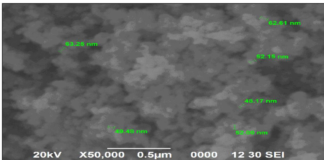
Fig.-2(b): SEM images of ZnO nanoparticles
