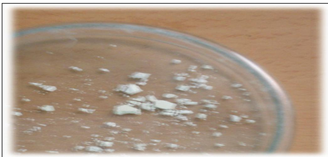
Fig.-1: Picture of synthesized Zinc Oxide nanoparticles
