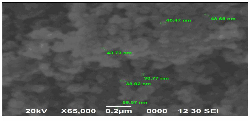
Fig.-2(a): SEM images of ZnO nanoparticles
